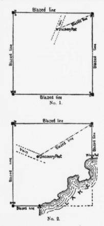
(4) The following diagrams are intended to illustrate the method of staking out a claim as mentioned in subsections 1 and 2.
