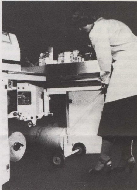
Refilling the Bag-O-Mat's paper supply mechanism, which is hidden under the attractive cabinetry, takes only a few seconds. The Bag-O-Mat is available with or without the computerized scanner for ringing in prices.
