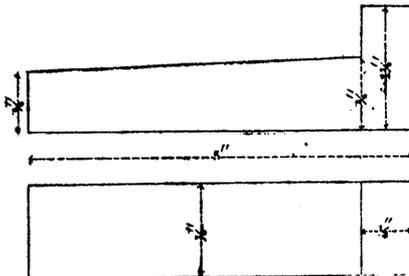
FIG. 2.—SKETCHES OF KEY FOR A WHEEL.
