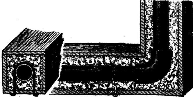
Fig. 5.—Method of Using Mineral Wool by Means of Wooden Boxes. Plan Well Adapted for Use of Pipes Exposed to the Weather.
