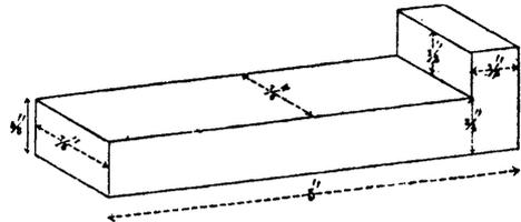
FIG. 3.—PERSPECTIVE SKETCH OF KEY FOR A WHEEL.
