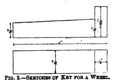
It will be seen at once that there are here two systems pursued. In the first (Fig. 1) the dimension figures are placed, when possible, or convenient, outside of the sketch and all standing one way. In the other (Fig. 2) the figures are placed as much as possible within the sketch and in each case at a right angle to the location of the dimension marked. The former is obviously the plainer and easier to read.
