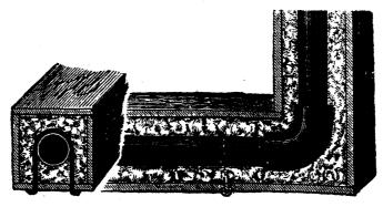
Fig. 5.—Method of Using Mineral Wool by Means of Wooden Boxes. Plan Well Adapted for Use of Pipes Exposed to the Weather.
