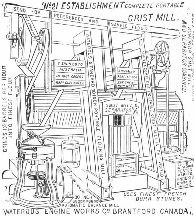
SEND FOR REFERENCES AND SAMPLE FLOUR. USES FINEST SILK BOIT CLOTH SUPERIOR SMUT MILL AND SEPARATOR COMBINED. GRINDS 1 1/2 BARRELS PER HOUR INTO FINEST FLOUR. WATEROUS STANDARD 30 INCH PORTABLE FLOURING MILL. 30 INCH UNDER RUNNER AUTOMATIC BALANCE MILL. WATEROUS ENGINE WORKS CO BRANTFORD CANADA.
