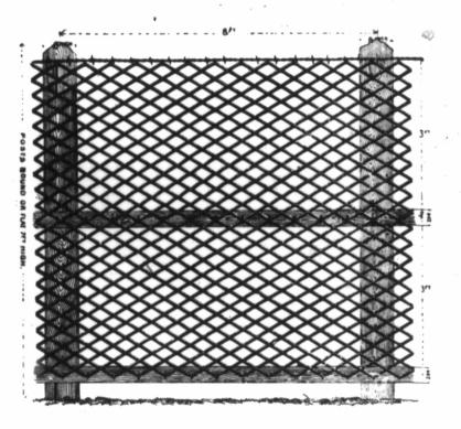
E ILLUSTRATE HERE a superior fence for railroad, orchard or cemetery needs. We' provide the Expanded Metal Sheets in 8 feet lengths, and these, if stapled securely to a simple framing, with barb wire at top, give for its strength the cheapest fence that can be procured for places where intrusions are to be guarded against. The height shown is 6 feet, but anything up to 8 feet is available without splicing. We provide the Expanded Metal sheets. See General Price List, page 16.
