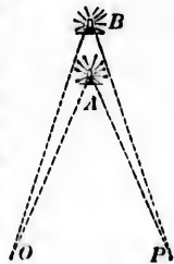
FIG. 47.—Diagram illustrating parallax.
