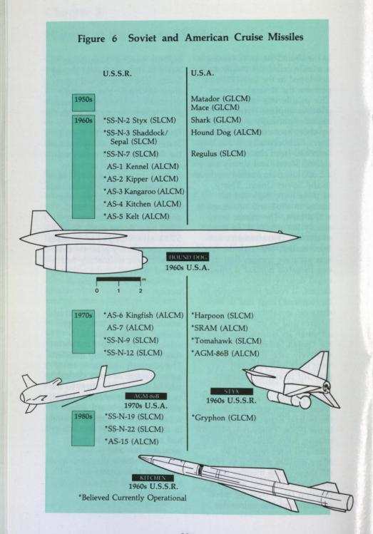
A number of anti-ship cruise missiles were developed with ranges of tens to hundreds of kilometres first by the Soviet Union in the 1960s, and then also by the United States in the 1970s. At this time, it was not practical to develop cruise missiles with longer ranges because, among other things, there was no way to detect ships at longer ranges.
