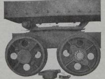
This view shows the oil or grease retaining cap removed to show the Roller Bearings supplied on our Mine Cars.
