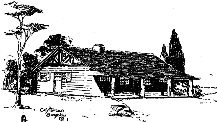
Design No. 7.—A craftsman bungalow, sheathed with boards 8 x 10 inches wide, 3/4 of an inch thick, laid like clapboards. Note the truss of hewn timber in the gable, which not only forms a decorative feature, but gives added support to the roof.
