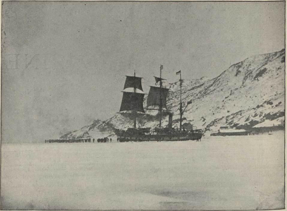
S.S. "MASTIFF" WORKING BY STEAM, SAIL, AND TOW-LINE THROUGH THE HARBOUR ICE.
