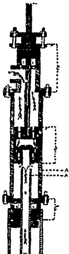
24041 Yates' Force Pump for forcing fluids long distances, extinguishing fires and other purposes.
