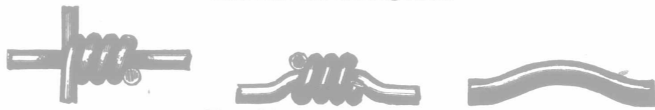
Hinge Joints and Tension Curves.
