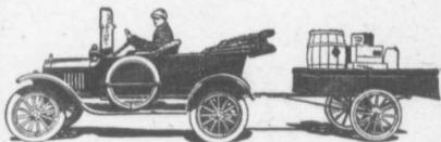
The Fox Trailer is constructed on an all-steel frame. This insures rigidity and durability. The tires are of solid rubber mounted on regular automobile wheels. The draft is direct from the trailer axle. This gives an even pull without bumping.
