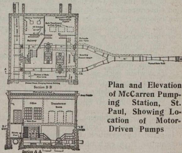
Plan and Elevation of McCarren Pumping Station, St. Paul, Showing Location of Motor-Driven Pumps
