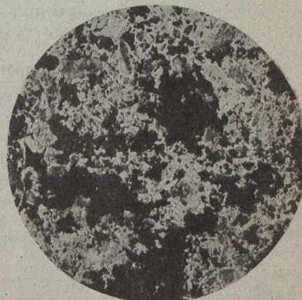
Fig. 2—Sample of Concrete from Vancouver Sewer Pipe, Magnified Two Diameters—Black Areas Indicate Voids
