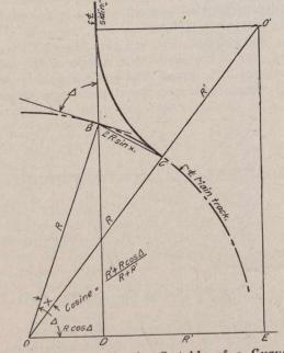
Fig. 4.—A Siding from the Outside of a Curved Main Track.
