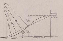
Fig. 1.- A Siding Parallel to the Tangent Main Track.
