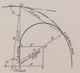
Fig. 5.—A Siding from the Inside of a Curved Main Track.
