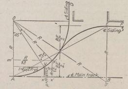
Fig. 2.—A Siding Parallel to or at Right Angles to the Tangent Main Track.
