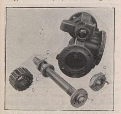
Fig. 1. A 14-in. expanding self feeding reamer.
