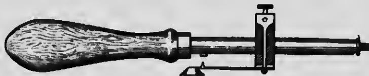
FIG. 51.—ELECTRODE HANDLE FOR TESTING WITH "CLOSING KEY."
