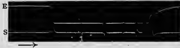
FIG. 33.—IRREGULAR DISCHARGES, DUE TO FAULTY ACTION OF INTERRUPTER.
