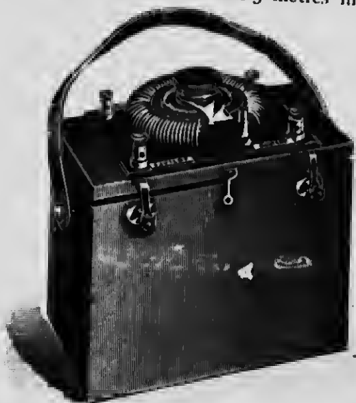
FIG. 64.—ACCUMULATOR FOR LAMPS AND CAUTERIES.
