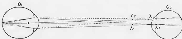
FIG. 234.—Showing the course of the emergent rays at the point of reversal. So long as \lambda_1 is in the pupillary area of O_2 , the pupil of O_1 appears uniformly illuminated, and there is no shadow. Directly \lambda_1 passes to \lambda_2 the whole of the light is cut off, so that the pupil of O_1 becomes completely dark.
