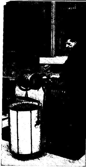
Hoisting head revolves. Can be deposited on sidewalk without lifting.
