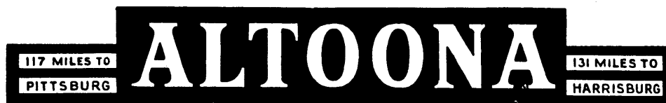
Style no. 3, as used on the Pennsylvania Railroad. White letters on black ground. This sign is 12 ins. high by 6 ft. long. Length varies with number of letters in name of station.
