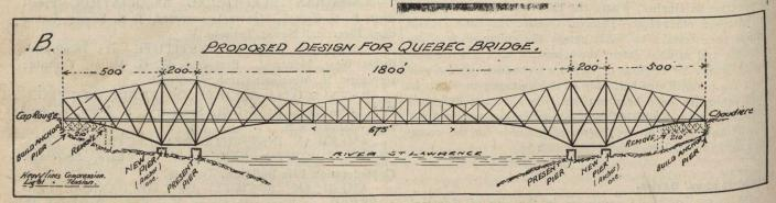
cannot be overestimated—it is a design especially providing for erection stresses, a feature lacking in the original.
