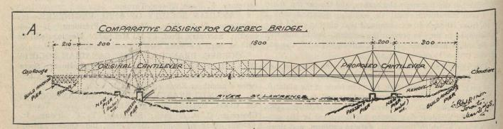
same length as in original design, and also the suspended span. This would bring the ends of anchor arms approximately on the land abutments. To carry out this plan, the approach spans of 210 feet each must be eliminated. These approach spans could be cut out, removed to new site and erected at probably one-third of their original cost; or possibly lowered intact on blocking to tide water, and towed on scows to some convenient site.
