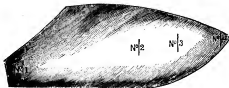
414— Morley's Improved Mould Board for Ploughs.
