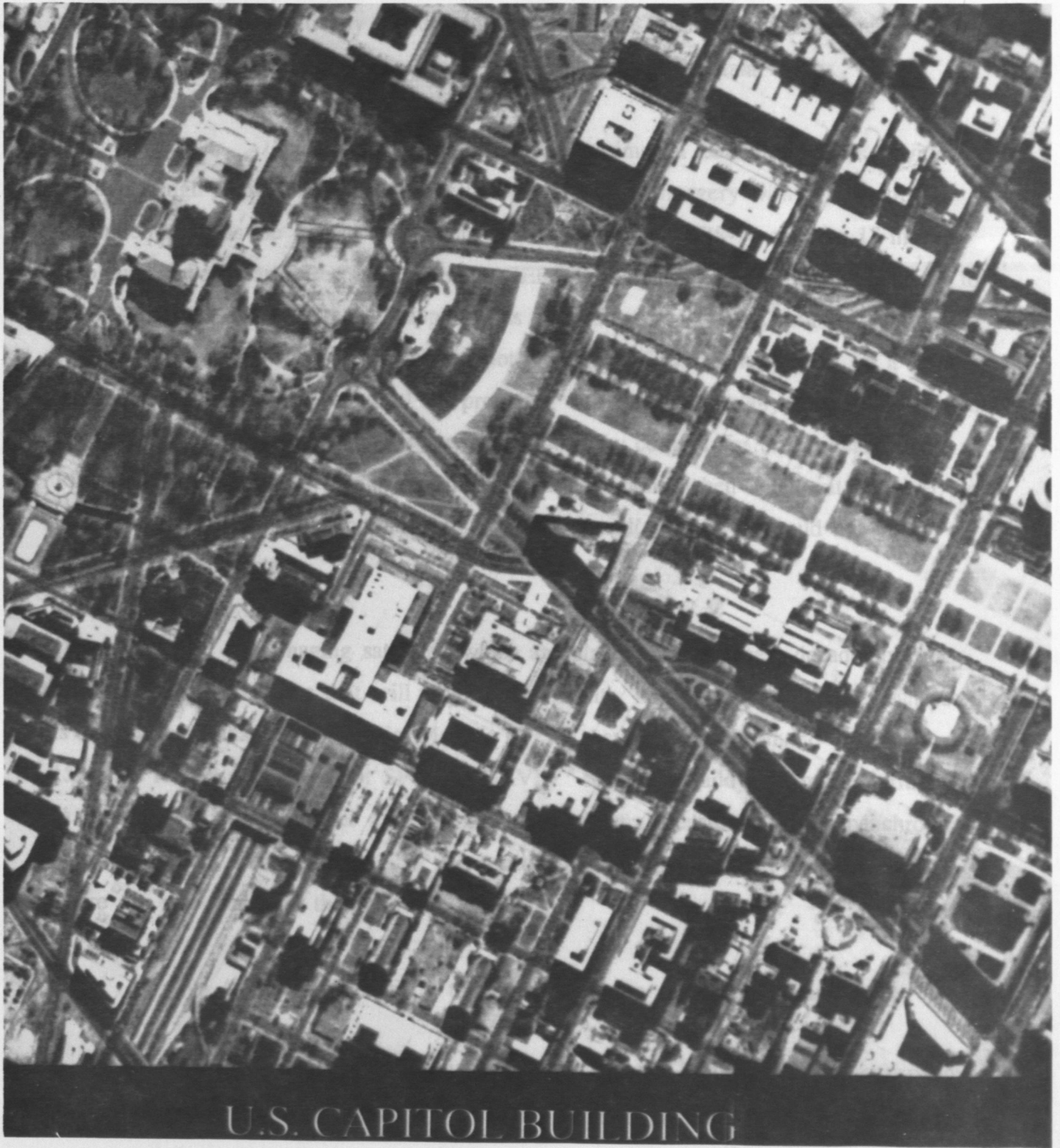
Figure 1. Recently high resolution Russian imagery has become commercially available. This KVR-1000 image of the Washington area has approximately two meter spatial resolution and has redefined the possible uses of commercial satellite imagery.
