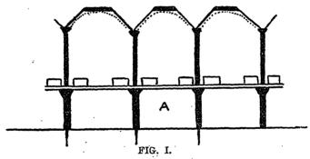
Transverse vertical section through series of wards to show method of lighting from above. The basement A is utilised to carry the ventilating shafts and heating apparatus.
