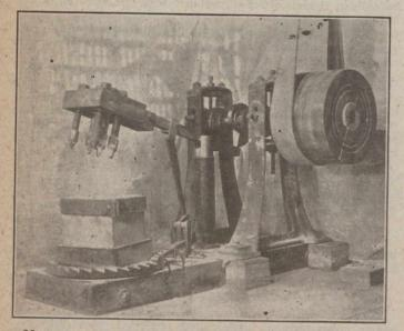
MACHINE FOR GENERATING IMPACT STRESSES CLOSELY RESEMBLING THOSE CAUSED BY TRAFFIC, THUS DETERMINING WEAR-RESISTING VALUES OF VARIOUS AGGREGATES
