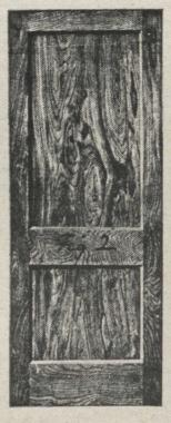
The type of door shown in Fig. 2 furnishes an excellent opportunity to show off good veneer work, especially in panels. It consists of two large panels, the top one full width running practically two-thirds of the length, and the
