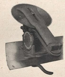
This is a new tool for the circular saw operator It clamps the circular saw while the filer is filing it.
