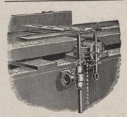
Jointer Guard Dotted line shows it at side of machine for rabbiting.
