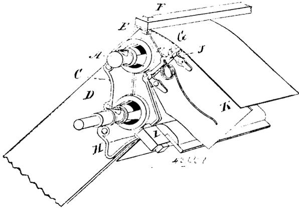
locked, substantially as and for the purpose set forth. 2nd. A metal plate arranged to support the roller spindles, and having cast integral with it a lug to carry the cross bar for the deflector, a lug to support the cross bar of the binder deck, and a flange to form one-half the hinge for the header board, substantially as and for the purpose specified.
