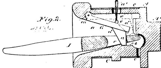
guide plates projected oppositely at the sides of said case, a latch block hinged within the front portion of the draw-head, a depending tongue thereon adapted to seat in a groove in the conical recess, and a device on the front of the car adapted when manipulated, to raise the latch block, substantially as described.
