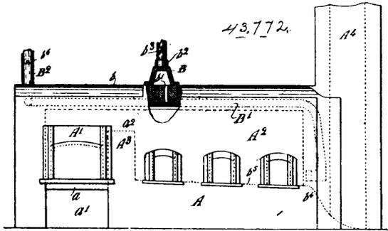
communicating with the rear portion of said puddling or heating chamber near its bottom and pipes or flues extending along the walls of the furnace and communicating with said last named ports or passages, substantially as specified.
