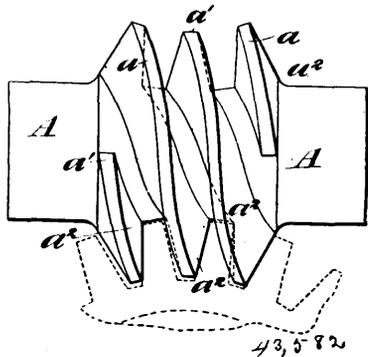
axis of the worm, and the teeth on the worm wheel, having their contact sides formed in a compound curved plane, having a general oblique direction across the face of the wheel to correspond to the face of the worm tooth, substantially as set forth.
