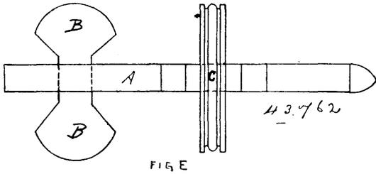
composed of material having an appearance of a rigid non-compressible substance, two heads or enlarged portions located at opposite ends of the restricted portion, and a second piece formed with an aperture corresponding to the size of the restricted portion and adapted to be engaged over the head when the same is compressed, substantially as described.
