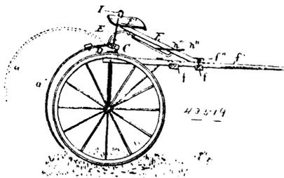
rods *g* and *h*, the bow *E*, and the rake head *C*, with the teeth *a*, all as and for the purpose described.
