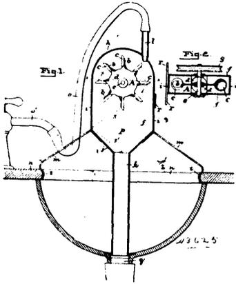
turn or twist, and cups on the tangs, a vertical inlet nozzle entering the case top, and a spacious chamber *p* in the case below the wheel, as shown and described. 2nd. A portable water motor having a vertical case *A*, provided with a vertical discharge pipe in its lower end, a vertical wheel in the case and two spring arms *m*, each attached to the case at a side opposite the other said arms, having at their free end an ogee curve or bend *t*, as and for the purpose set forth.
