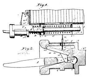
guide plates projected oppositely at the sides of said case, a latch block hinged within the front portion of the draw-head, a depending tongue thereon adapted to seat in a groove in the conical recess, and device on the front of the car adapted when manipulated, to raise the latch block, substantially as described.
