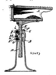
stantially as and for the purpose specified. 3rd. The combination of the stationary standard, formed with an annular recess in its interior, the vertically movable support sliding loosely in said standard, a friction or clamping spring consisting of a split ring located within the annular recess in the standard and adapted to press or bear against the movable support and the binding screws, substantially as set forth.
