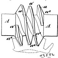
axis of the worm, and the teeth on the worm wheel, having their contact sides formed in a compound curved plane, having a general oblique direction across the face of the wheel to correspond to the face of the worm tooth, substantially as set forth.
