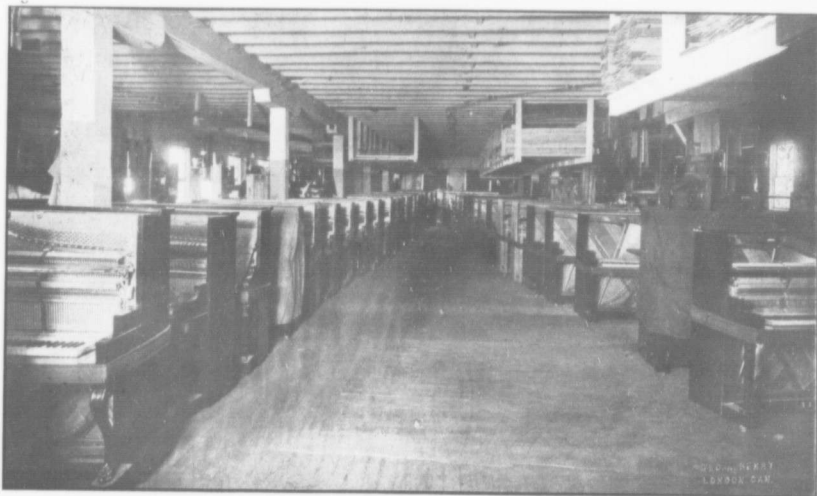
No. 13. View of a portion of Piano Department showing the long lines of Pianos allowed to stand for seasoning.
