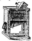
THE CLINTON CORN SHELLER, with iron hopper, simply and firmly secured with double spring to suit all sized ears, with balance wheel playing inside, and safe from injury, is best adapted to northern corn, and warranted the most perfect article in the market. With it a bushel can easily be shelled in five minutes.
