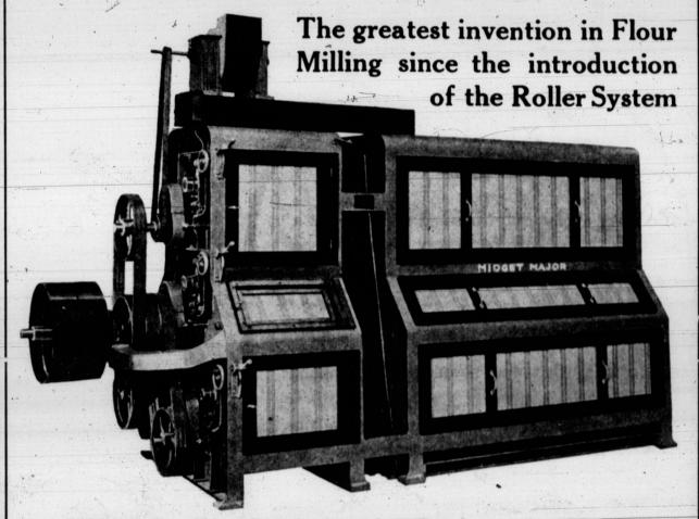
Made in Two Sizes, Capacity 25 and 45 Barrels per day (24 hours)
