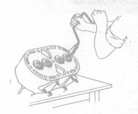
Fig. 2—Grinding Valves in Valve-in-head Type of Engine. With acknowledgements to the I. H. C.
