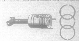
Fig. 3—Replacing Piston Rings. Note strips of tin used for sliding rings to the grooves.
