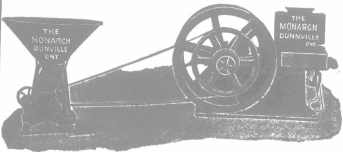
8 h.-p. Hopper Cooled Engine with 10-inch Grinder.
