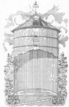
1.—Section of stave silo—a a, drain; b, foundation; c, ground floor; d, cement floor; l, l, hoops.
