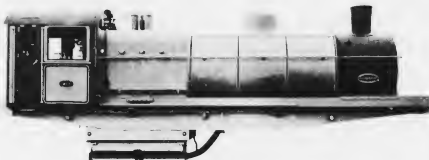
Boiler and Frame.
