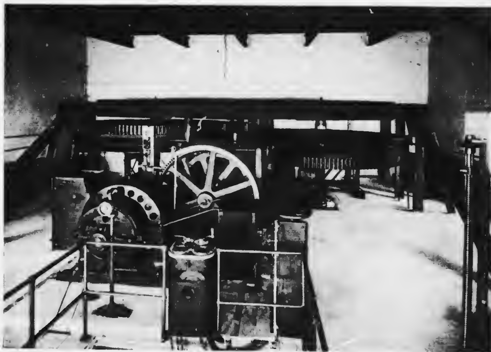
INTERIOR OF THE DRIVING STATION, WETTERHORN AERIAL RAILWAY. Showing the two great winding drums driven by a 45-horse-power electric motor.
