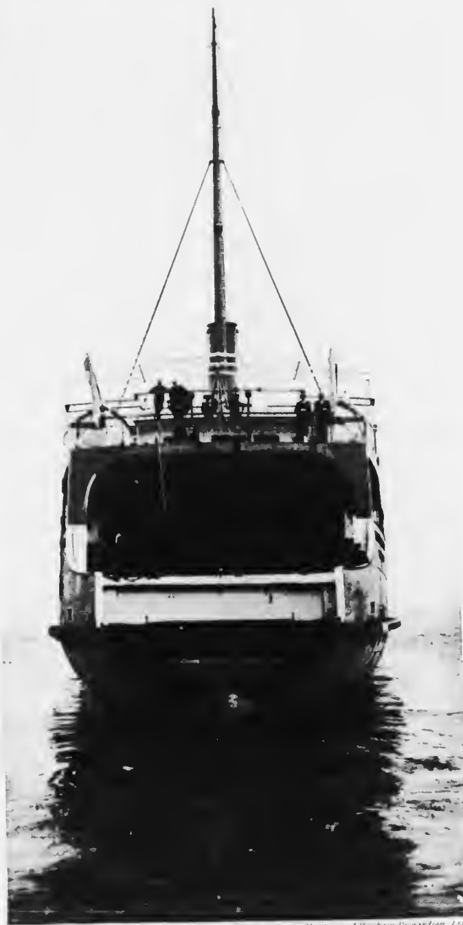
Photograph by permission of Swan, Hunter, and Wigham-Rigartson, Ltd. STERN VIEW OF THE DROTTNING VICTORIA. Showing the car deck and berthing arrangements.
