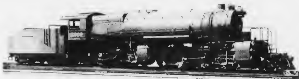
THE "BIG BULL-MOOSER" OF THE GREAT NORTHERN RAILROAD, U.S.A. This Baldwin-Mallet compound locomotive (2-8-0, 0-8-0) is used for the heavier class of traffic—passengers and goods—among the mountains. Total weight, with tender, 300 tons.
