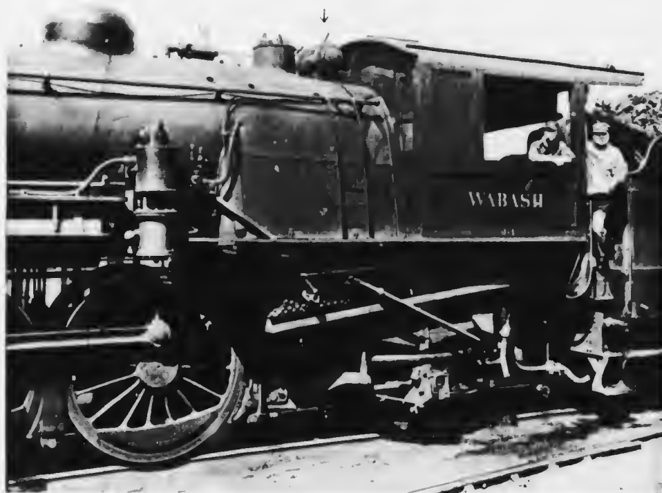
A LOCOMOTIVE FITTED WITH DYNAMO (MARKED BY ↓) FOR HEADLIGHT The dynamo is turbine-driven and generates current for the headlight and three incandescent lamps in the cab.
