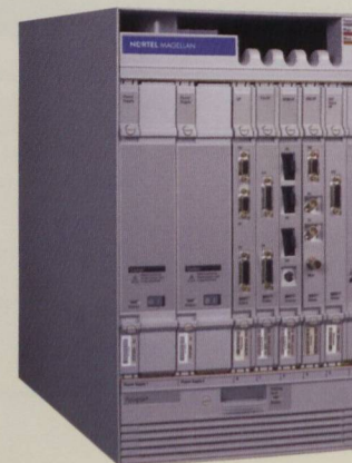
A major Canadian telecommunications company is Nortel Networks Japan. Displayed is Nortel's "Passport 6400" series network switch.
