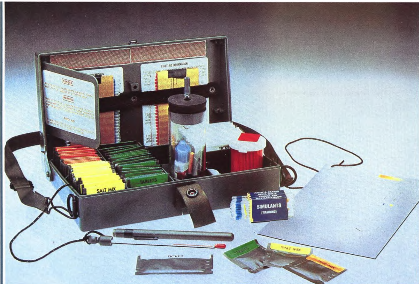
Chemical agent water testing kit M272.
