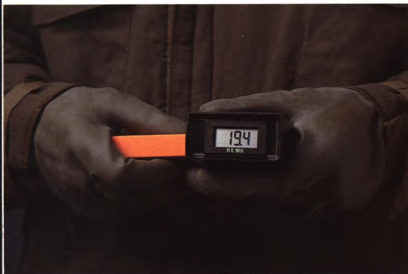
The Reader reads its own dose level or that of the Badge.
