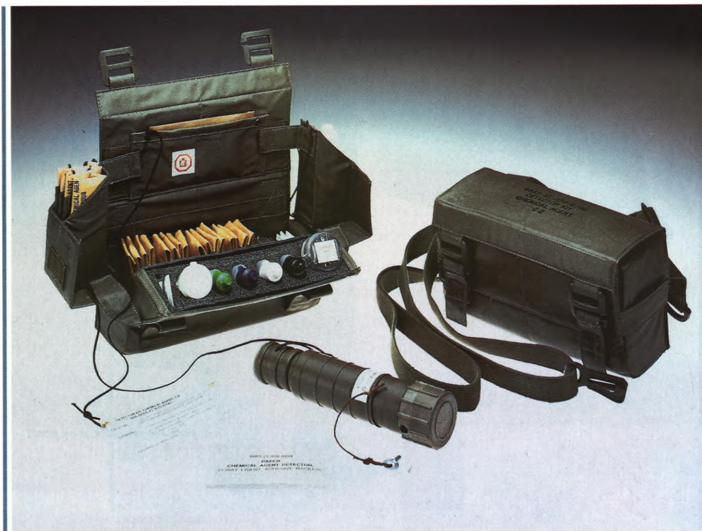
Chemical agent detector kit C-2 open on the left, displaying contents; and closed on the right showing carrying strap. Note the air sampling pump in the foreground.
