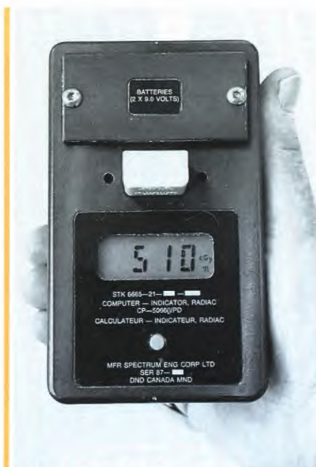
With the locket in place, the reader provides accurate dose readouts on its LCD display.
