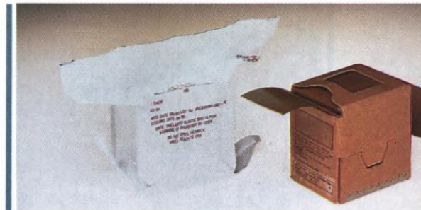
Chemical agent liquid detector M9.
