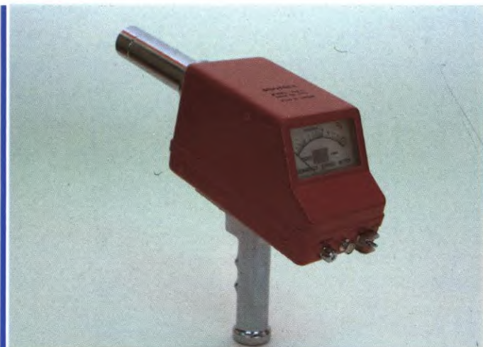
Emergency high range gamma survey meter and dose integrator, Model 189C.
