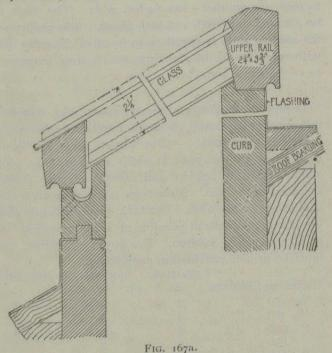
other, so that the sash will have an inclination of about 2 inches to the foot. In flat toofs the frame or curb may be set on top of the roof. Fig 167a shows another detail, which is in some respects superior for large skylights."
