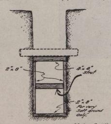
Fig. 3,-Protection Against Mains Settling.
