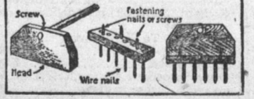
The Construction of a Garden Rake Head in Which Nails Are Used for the Teeth.
