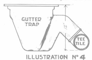
Showing gutter trap.
