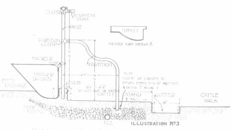
Ideal measurements, showing best sizes, rounded corners and stone filling.
