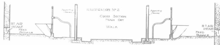
Showing two rows of cow stalls and relative positions of galvanized steel stalls, columns, mangers, water bowls, passages and gutters.
