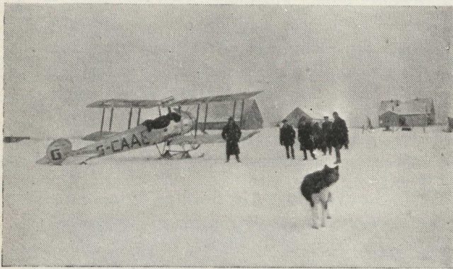
Avro Aeroplane, Flown by Canadian Aerial Services' Pilots, just after landing at Moose Factory in the Far Northland. Note sled runners replacing wheels in landing gear.
