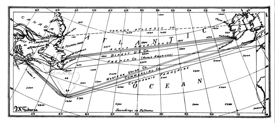
—— Telegraph lines and cables in operation. --- do. projected.
