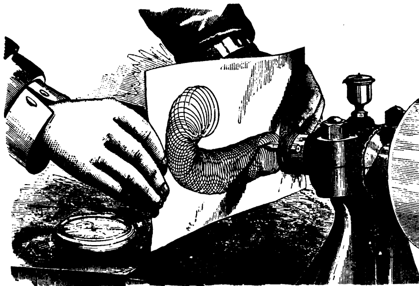
SIMPLE MODE OF ASCERTAINING THE REVOLUTIONS OF A SHAFT.
