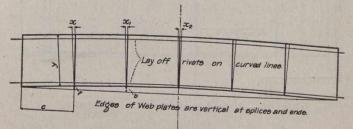
Fig. 8.-Plate Girder With Five Web Splices.
