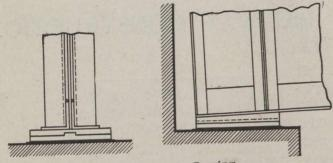
Fig. 1.-Sliding Bearing.
