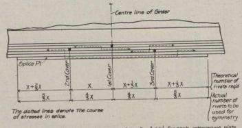
Number of riveto required to oplice cover plate=X Add's for each intervening plate Theoretical number of riveto required=5X+\$X Number of riveto required for symmetry=GX
