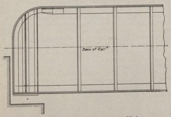
Fig. 9.-Curved End for Through Cirder.
