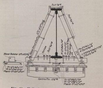
Fig. 11.-Method of Loading Cirder on Flat Car.
