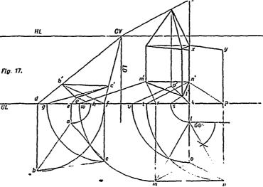
ward LMP, to p, t', 2' and r, and from these erect perpendiculars to cut lines from n and o to CV in 3', 4', 5' and 6'. Join these and thus complete the figure.
