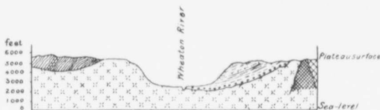
Fig. 1. Diagrammatic section showing the plateau-surface truncating the different rock formations, and cut by Wheaton River valley.
