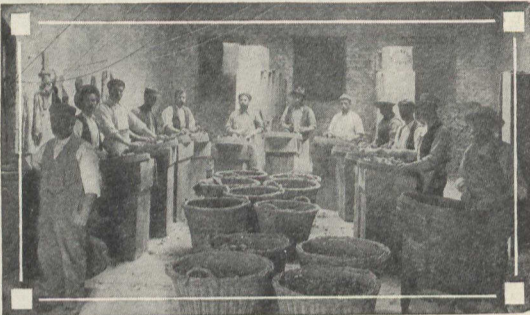
Sorting and grading gums. The first careful step in varnish-making. Gums come chiefly from New Zealand, Africa and India.
